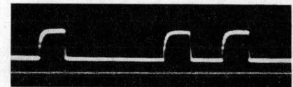
Fig. 2(b). Controls on individual generator can be used to vary individual pulses in train. Second and fifth pulses have been reduced to zero amplitude.
